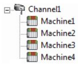
Channel1 Machine1 Machine1 Bach device appears under a single channel. In this configuration, the driver must move from one device to the next as quickly as possible to gather information at an effective rate. As more devices are added or more information is requested from a single device, the overall update rate begins to suffer.
