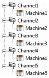
Channel1 Each device has now been defined under its own channel. In this new configuration, a single path of execution is dedicated to the task of gathering data from each device. If the application has fewer devices, it can be optimized exactly how it is shown here.
