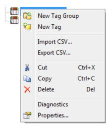
Tag groups can be added at any level from the device-level down, and multiple tag groups can be nested together to fit the application's needs. As seen in the OPC Quick Client dialog above, the fully qualified OPC item path is "Channel1.Device1.Machine1.Cell1.Tag1". For this OPC item, "Machine1" and "Cell1" segments are nested tag groups.
